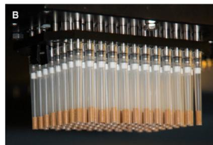
**Figure 2.** MiniPrep PhyTip® Columns for Plasmid DNA Purification
